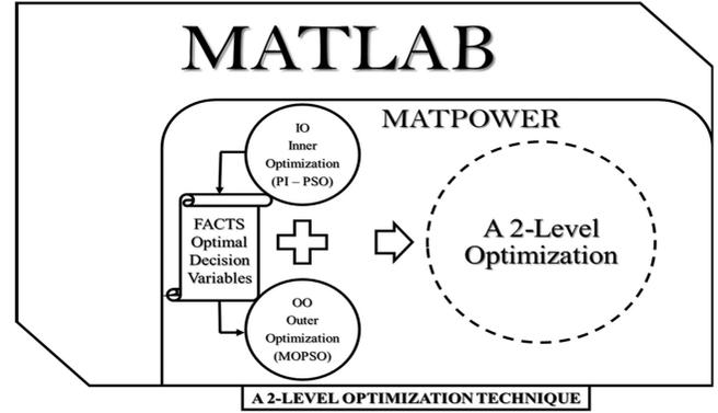
**Fig. 1.** Schematic of the bi-level optimization for FACTS–DG coordination. FACTS, flexible alternating current transmission systems; DG, distributed generation.
