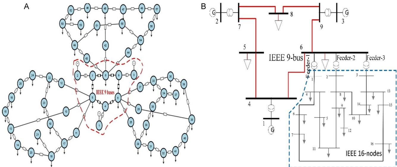
Fig. 3. Integrated test network. (a) Topology in steady-state AC network visualization. (b) A simplified one-line diagram.
