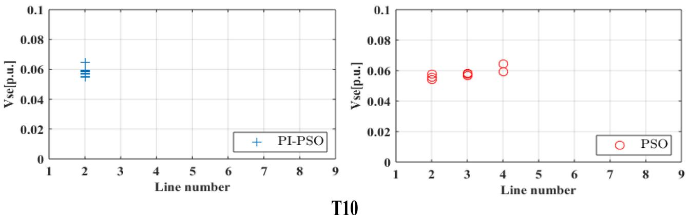
Fig. 8. A typical plot of particles’ positions versus  $V_{se}$  for PI-PSO and PSO with SSSC. PI, performance index; PSO, particle swarm optimization; SSSC, static synchronous series compensator.
