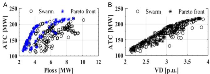
**Fig. 11.** Slices of Pareto plot for transaction T1 under TCSC–PQ<sub>DG</sub>. (a) ATC versus power loss ( $P_{loss}$ ) (b) ATC versus voltage deviation ( $V_D$ ).
