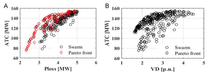
**Fig. 12.** Slices of Pareto plot for transaction T2 under SSSC–PQ<sub>DG</sub>. (a) ATC versus power loss ( $P_{loss}$ ) (b) ATC versus voltage deviation ( $V_D$ ).
