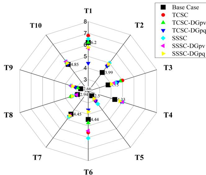
**Fig. 5.** Performance of FACTS-DG coordination under power losses. FACTS, flexible alternating current transmission systems; DG, distributed generation; SSSC, static synchronous series compensator; TCSC, thyristor-controlled series compensator.
