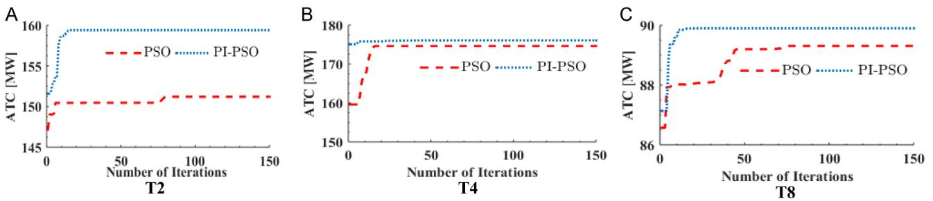
Fig. 7. Convergence curve of PI-PSO and PSO for ATC enhancement with SSSC. ATC, available transfer capability; PI, performance index; PSO, particle swarm optimization.
