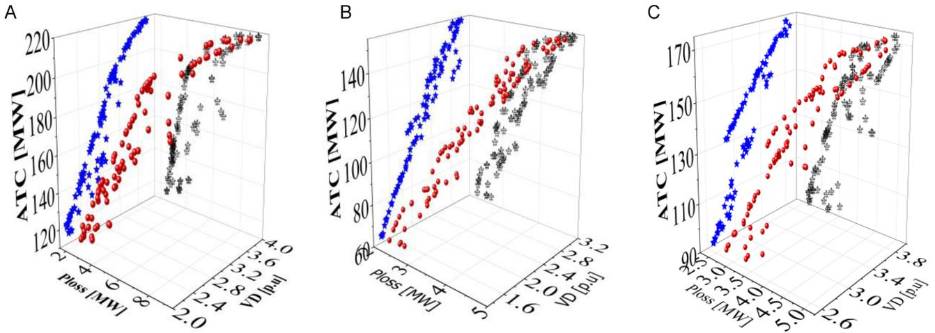
**Fig. 9.** Pareto front plot for different transactions under TCSC–DG coordination. (a) T1 TCSC–PQ<sub>DG</sub> (b) T2 TCSC–PV<sub>DG</sub> (c) T3 TCSC–PV<sub>DG</sub> ATC, available transfer capability; PQ, reactive power; PV, real power; TCSC, thyristor-controlled series compensator.
