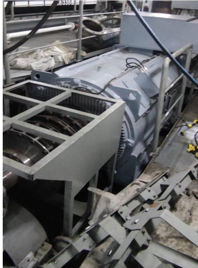
Fig. 4. Overview of a shaft generator in a ship.
